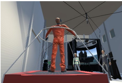
Impression of the Maritime eXperience Lab (MX Lab) with motion platform, treadmill, cable robot and Fast Small Ship Simulator (FSSS).
